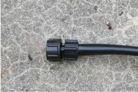
Above. Place the end of the hose fitting into the poly tubing and twist into place.
