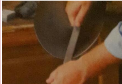
Use an 8 in, medium flat mill file. Push down away from your body and across the blade of shovel until sharpen.
