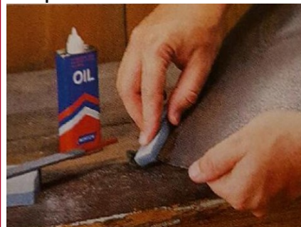
Check the rough edge on back of shovel called a "burr". With a few small drops of oil on blade, gently rub a fine grit grinding stone over it until the burr is gone.
