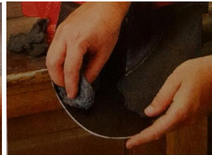
Wipe entire blade with steel wool and add more oil. Any good oil, machine or vegetable, will do to keep surface from rusting. Leave heavy coat of oil if storing tool, wipe clean if headed to the garden.
