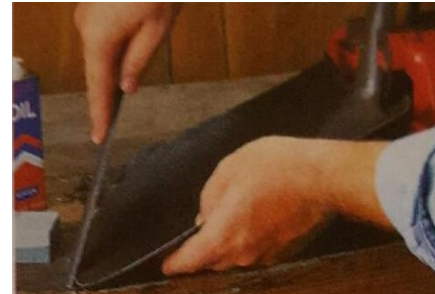
Check the blunt bevel on back of blade, this is best on tools for tough digging.
